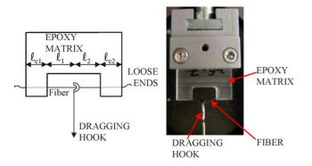
Fig. 1. Schematic diagram of drag out specimen and picture of spectra/epoxy specimen in the tensile holder.
