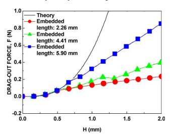
Fig. 3. The drag-out force F as measured with different embedded lengths. The predicted theoretical line (Eq. (4) or, equivalently, Eq. (6)) is shown for comparison.
