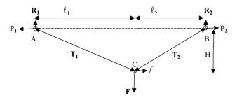
Fig. 2. Force equilibrium for the drag-out configuration.
