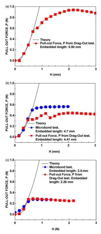
Fig. 4. The horizontal force P as measured for different embedded length (a) 5.9 mm (b) 4.41 mm (c) 2.26, in comparison with Eq. (5) and with traditional microbond test.
