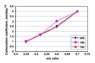
Fig. 5 Effect of cement content (i.e. different levels of water contents of about 160, 180 and 200 kg/m<sup>3</sup> of concrete) on carbonation coefficient in accelerating conditions
