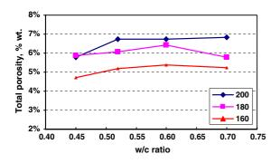
Fig. 2 Effect of cement content (i.e. different levels of water contents of about 160, 180 and 200 kg/m<sup>3</sup> of concrete) on total absorption
