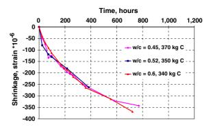
Fig. 14 Effect of w/c on shrinkage of concretes having a roughly similar cement content of about 350 kg/m<sup>3</sup>
