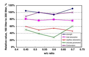
Fig. 10 The effect of cement content on the relative values of strength, total absorption, capillary absorption, chloride penetration and carbonation for mixtures with about 160 kg/m<sup>3</sup> water content relative to mixtures with about 200 kg/m<sup>3</sup> of water, i.e. cement content reduction of about 20%
