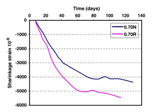
Fig. 9 The effect of admixture content and type on the shrinkage of w/c = 0.70 paste (0.70 N—without admixture; 0.70R—with Rheobuild 700 admixture)
