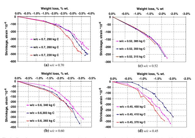
Fig. 6 Effect of cement content on shrinkage—weight loss curves of concretes having the same w/c ratio but differing in their cement content. (a) w/c = 0.70, (b) w/c = 0.60, (c) w/c = 0.52, (d) w/c = 0.45)
