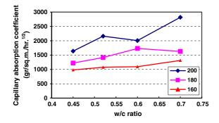
Fig. 3 Effect of cement content (i.e. different levels of water contents of about 160, 180 and 200 kg/m<sup>3</sup> of concrete) on capillary absorption coefficient
