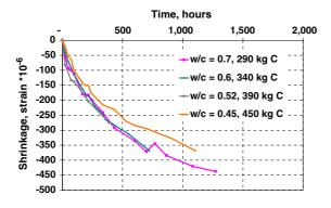
Fig. 7 Effect of w/c on shrinkage-time curves of concretes having a similar water content of about 200 kg/m<sup>3</sup>
