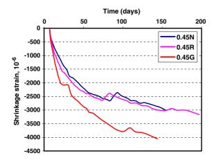
Fig. 8 The effect of admixture content and type on the shrinkage of w/c = 0.45 paste (0.45 N—without admixture; 0.45R—with Rheobuild 2000 admixture; 0.45G—with Glenium admixture)
