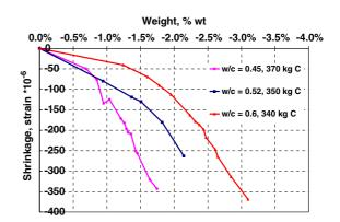
Fig. 13 Effect of w/c on shrinkage—weight loss curves of concretes having a roughly similar cement content of about 350 kg/m<sup>3</sup>
