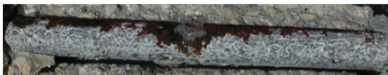
Fig. 9. Rebar with worm-like deposits on its non-corroded part.
