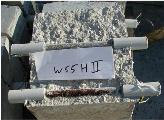
Fig. 6. Split specimen a few months after corrosion initiation.
