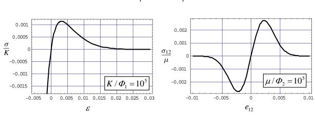
**Figure 2.** Left: Hydrostatic tension  $\sigma/K$ . Right: Simple shear  $\sigma_{12}/\mu$ .
