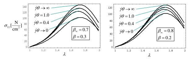
Figure 5. Uniaxial tension for various strain rates.
