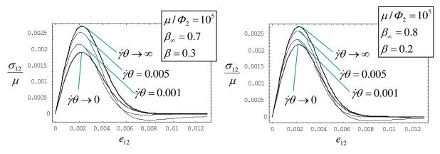
Figure 3. Simple shear for various strain rates.
