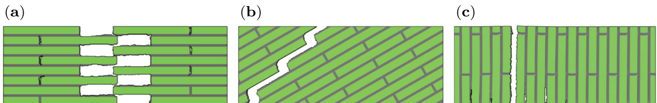
Fig. 8. Fractured samples for various offset designs with different inclination angles: (a) \alpha = 0^\circ , (b) \alpha = 30^\circ , and (c) \alpha = 90^\circ .
