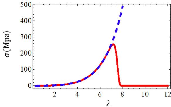
**Fig. 1** Cauchy stress versus stretch for uniaxial tension. Dashed line is for the model without failure and solid line is for the model with failure.
