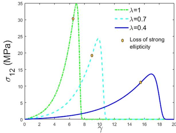
**Fig. 4 Shear stress versus amount of shear for various values of compression. Limit points designate the material strength and the elliptical markers on the curves indicate the loss of the strong ellipticity.**
